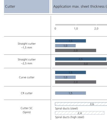
■ Steel (400 N/mm<sup>2</sup>) ■ High steel (600 N/mm<sup>2</sup>) ■ Aluminium (250 N/mm<sup>2</sup>) ■ Spiral ducts
