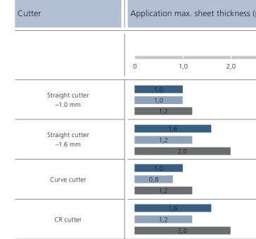
Steel (400 N/mm<sup>2</sup>) Stainless steel (600 N/mm<sup>2</sup>) Alu (250 N/mm<sup>2</sup>)
